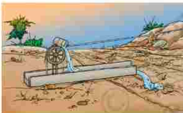
Fig. 1.4 (b) : Chain pump
